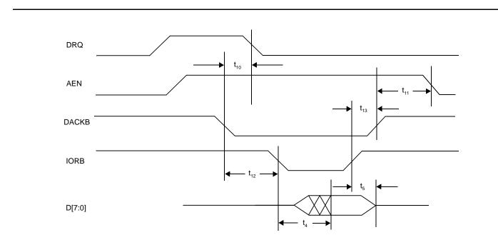
Figure 27 Compatibility Mode DMA Read Cycle
