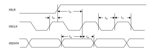
Figure 31 Serial Input Timing for I<sup>2</sup>S Interface
