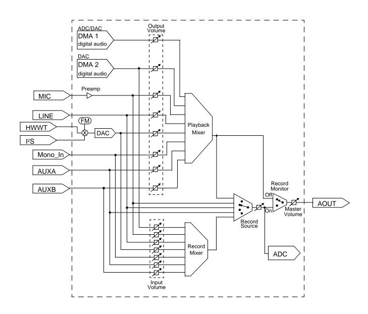
Figure 5 ES1869 Mixer Schematic Block Diagram
