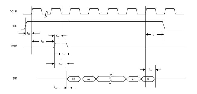
Figure 29 Serial Mode Receive Operation
