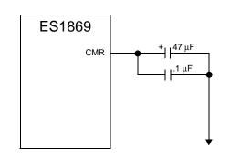
Figure 18 Reference Generator Pin Diagram
