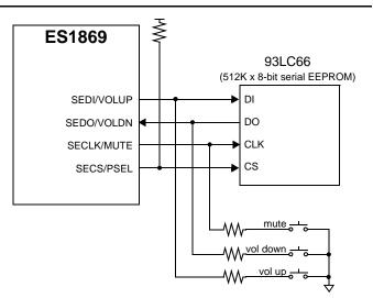
Figure 16 Serial EEPROM – Typical Application
