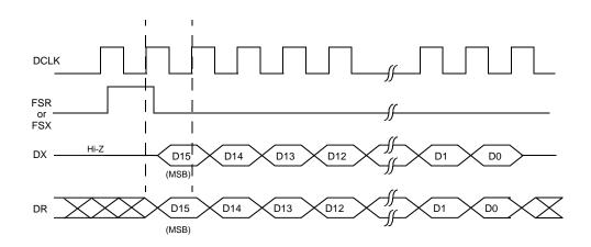
Figure 11 16-Bit Data, Positive Sync Pulse
