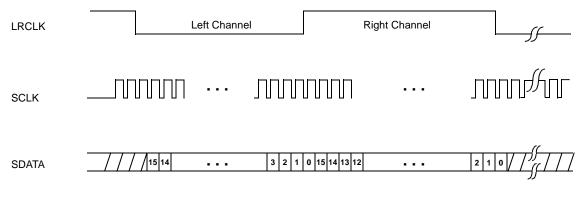
Figure 38 I<sup>2</sup>S Digital Input Format with 16 SCLK periods
