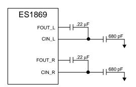
Figure 19 Switch-Capacitor Filter Pin Diagram
