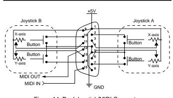
Figure 14 Dual Joystick/MIDI Connector
