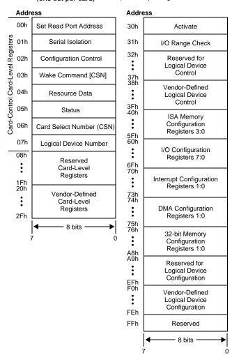
Figure 20 Configuration Register SeAccess to PnP Registers
