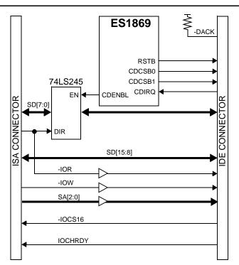
Figure 13 IDE Interface – Typical Application
