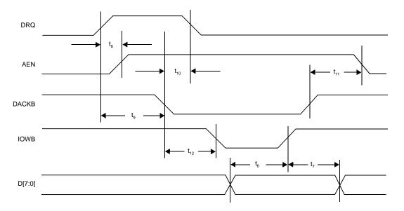
Figure 26 Compatibility Mode DMA Write Cycle
