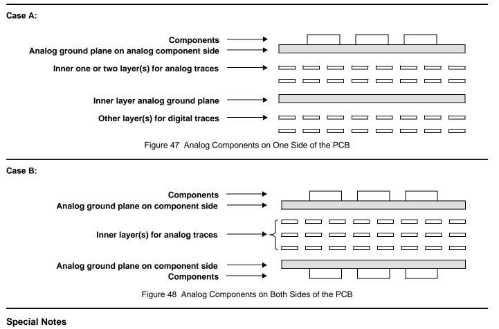
The analog traces should be placed as short as possible.
