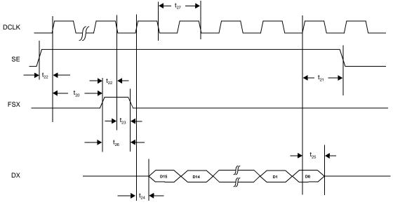
Figure 30 Serial Mode Transmit Operation
