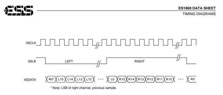
Figure 32 I<sup>2</sup>S Digital Input Format with 16 SCLK Periods
