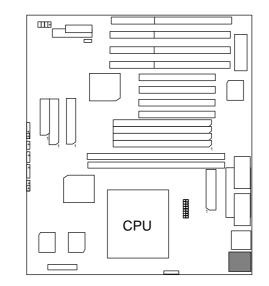
J1: CPU Cooling Fan Power Connector
